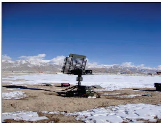
**Fig 4. Low Level Light Weight Radar ASLESHA**
