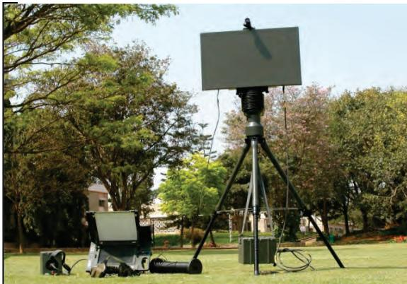
**Fig 2. Battery Field Surveillance Radar (BFSR)**
