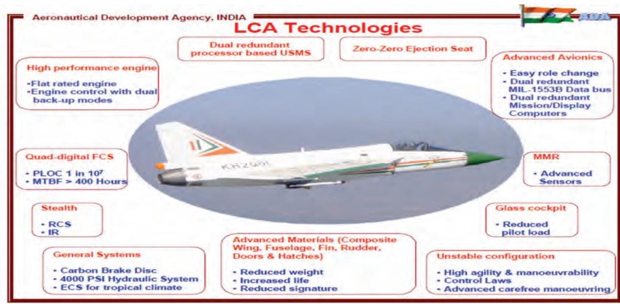
**Figure 1. LCA Technologies**
