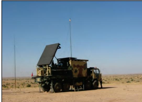
**Fig 3. Weapon Locating Radar (WLR)**
