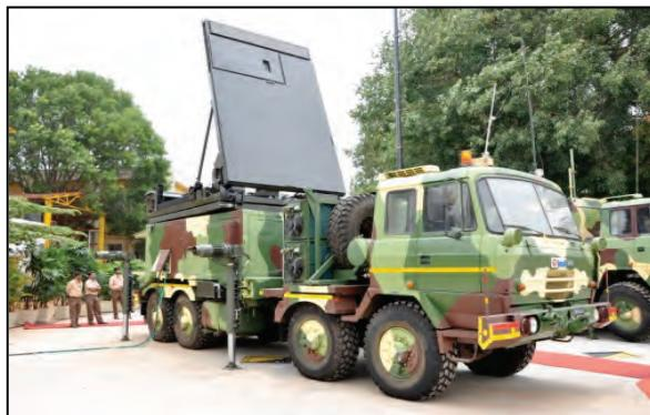
**Fig 7. Fire Control Radar – Troop Level Radar (TLR) for Army**
