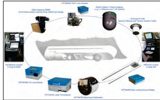
**Figure 2. Sensor Suite of the Octopod**
